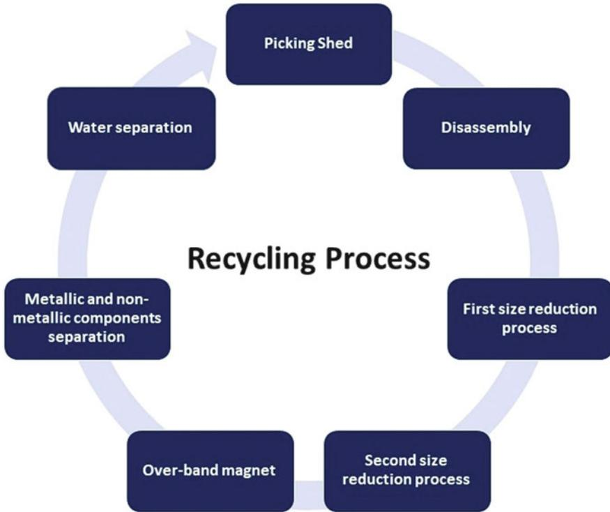
**Fig. 18.3** Different steps involved in e-waste recycling process
